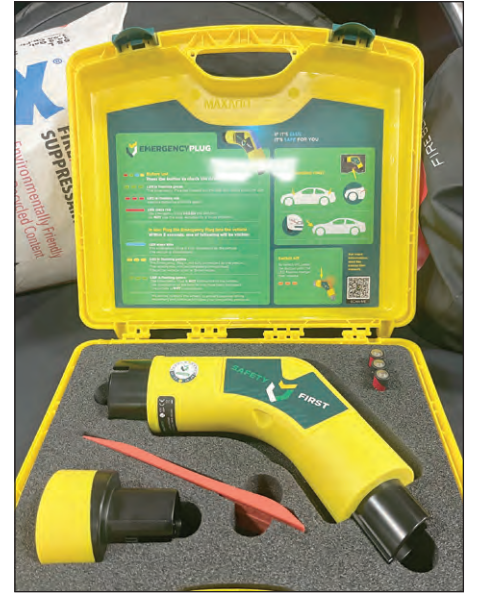
Turley Photos by Emily-Rose Pappas The Emergency Plug with its adapters to be used on electric vehicles.
